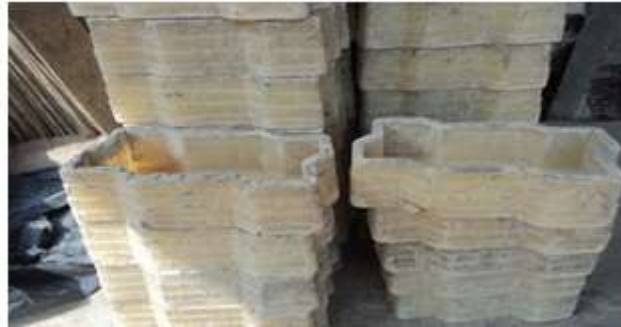
Figure 5: 80 mm thick rubber mould (Unipaver)
