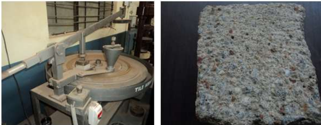
Figure 10: Abrasion resistance test on concrete paving blocks
