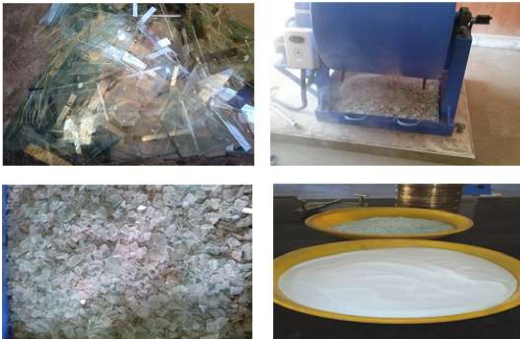
Figure 4: Collection and crushing of waste glass pieces and making powder (passing 600 micron sieve size)
